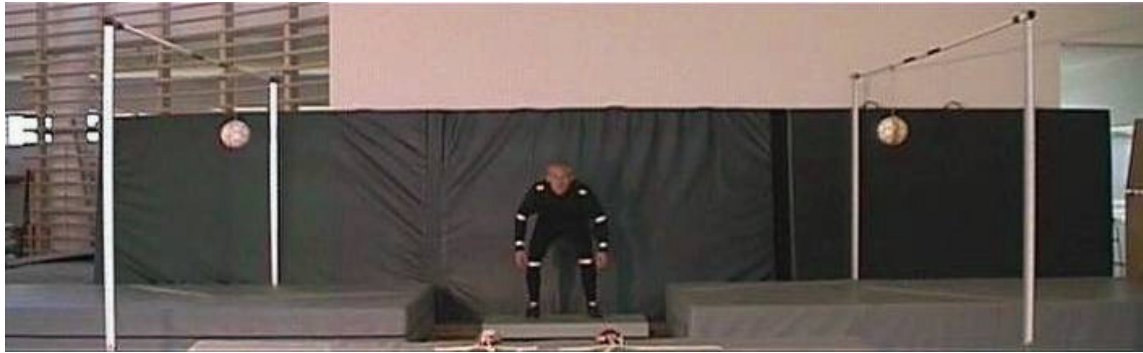
Figure 1 Setup for the reaction jump test. The two lamps, indicating to which side the subject should jump, are visible at the bottom of the picture.
