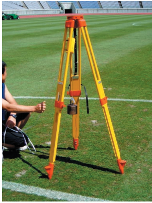
Figure 1 Impact hammer test apparatus.
